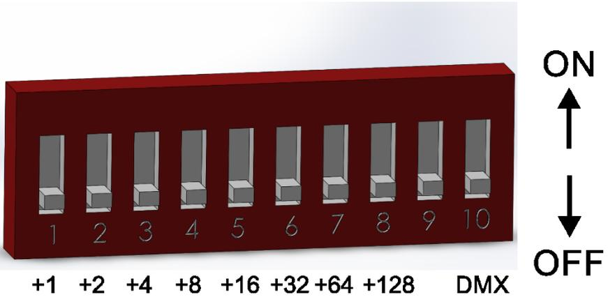
To reach a DMX address of 49 for example, turn switches 1, 5 & 6 to “On,”
